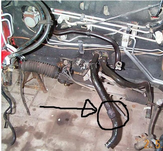
As you slowly fill the system water will start to come out of the first bleed valve when the water appears to have no air in it replace the bleed screw.
