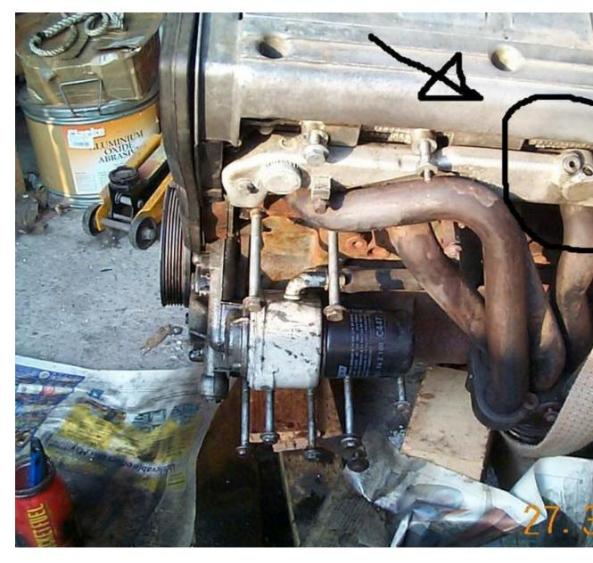
(on latter Coupes there may fitted a pipe from this location which goes to a connector back to the expansion tank an attempt to overcome the bleed problem.)
